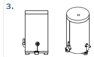
Fit the shell (black face on the outside) snuggly around the compressor. Place the cover on the top and seal the seams with soni VLC-01 adhesive tape.
